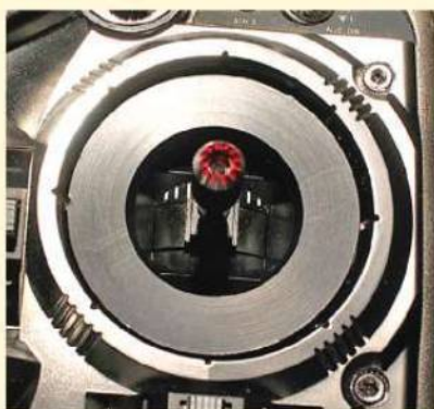
Mechanical cyclic rings will physically prevent the pilot from moving the cyclic stick into the trouble areas.
