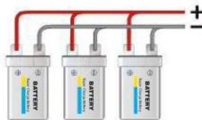
CELLS IN SERIES AND PARALLEL
